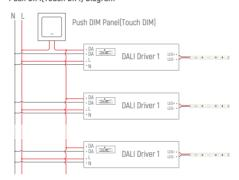
Remark: Only use open push button without indicator light. Maximum cable length between each Unit: 20 meters.
