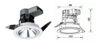
Description : Die-cast aluminum body. Matt white powder coating. Shiny reflector. Fixed downlight. Suitable for recessed T-bar or concealed ceiling. Available in white.
