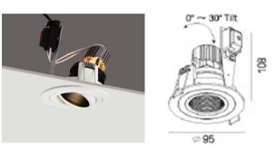
Description : Die-cast aluminum body. Sand white powder coating. Black reflector. Adjustable downlight. Suitable for recessed T-bar or concealed ceiling. Available in white.
